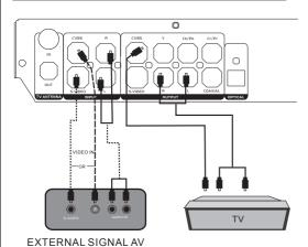
Connect your recorder with the S-Video cable, if the Signal source has an S-Video input. Do not connect the yellow video cable if using the S-Video cable.
